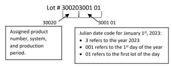
For traceability purposes, NuTek can determine the plant location, production line, and the date of manufacturing of the product from the lot number.
