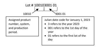
For traceability purposes, NuTek can determine the plant location, production line, and the date of manufacturing of the product from the lot number.
